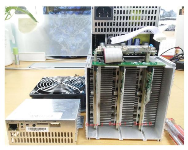
2) Remove the adapter plate and the copper bar fixed to the control panel as shown:
