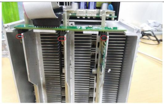
3) After the adapter plate is installed, install the copper bar. When the power busbar is connected to the hash board, the positive and negative poles of the copper bar cannot be connected incorrectly, and the screw pads of the fixed copper bar must be aligned with the edge of the copper bar, otherwise it may be possible to power on. The
