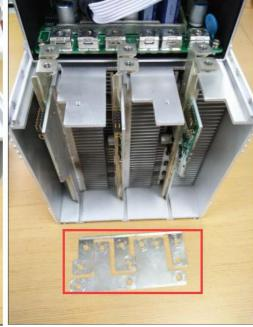
3) Extract the faulty hash board outward, as shown:
