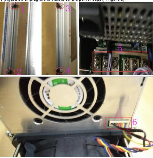
2) After the above operation is completed, gently pull out the power supply (do not pull out too long, the power control cable is still connected to the control panel), as shown in the figure:
