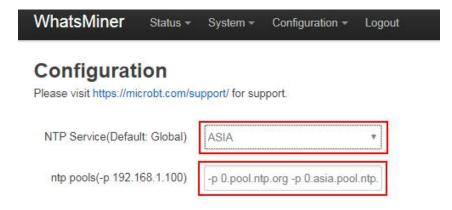
Default NTP server configuration: -p 3.asia.pool.ntp.org -p 2.cn.pool.ntp.org -p 1.cn.pool.ntp.org -p0.cn.pool.ntp.org Each -p is followed by the ntp server domain name or ip address, which can be modified or added according to the mine situation server address.
