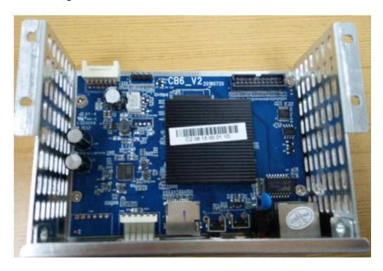
2) Insert the power control cable and the adapter board control cable into the corresponding slots on the control board, and then fix the bracket to the chassis with
