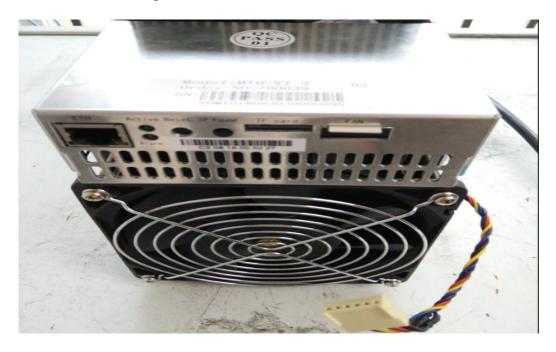
3) Plug the fan cable and the control board is installed.
