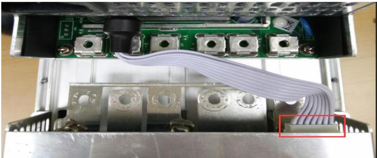
3) Unplug the power control cable on the control panel, remove the power supply
