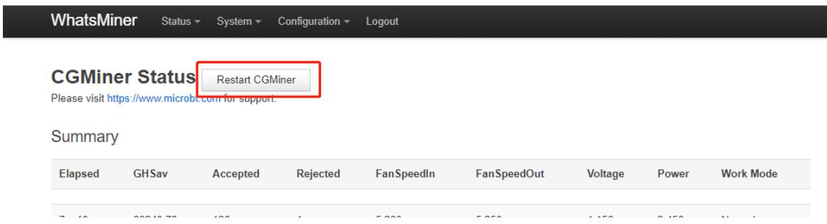
(4) Restart the control board and check whether the configuration modification takes effect. (If you do not choose to restart CGMiner, after the configuration is modified and saved, you can also restart the control board to make the configuration
