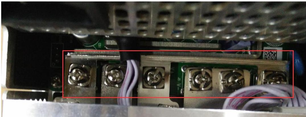
3) Finally, tighten the screws of the four fixed power supplies on the chassis, and the power supply is installed, as shown below:
