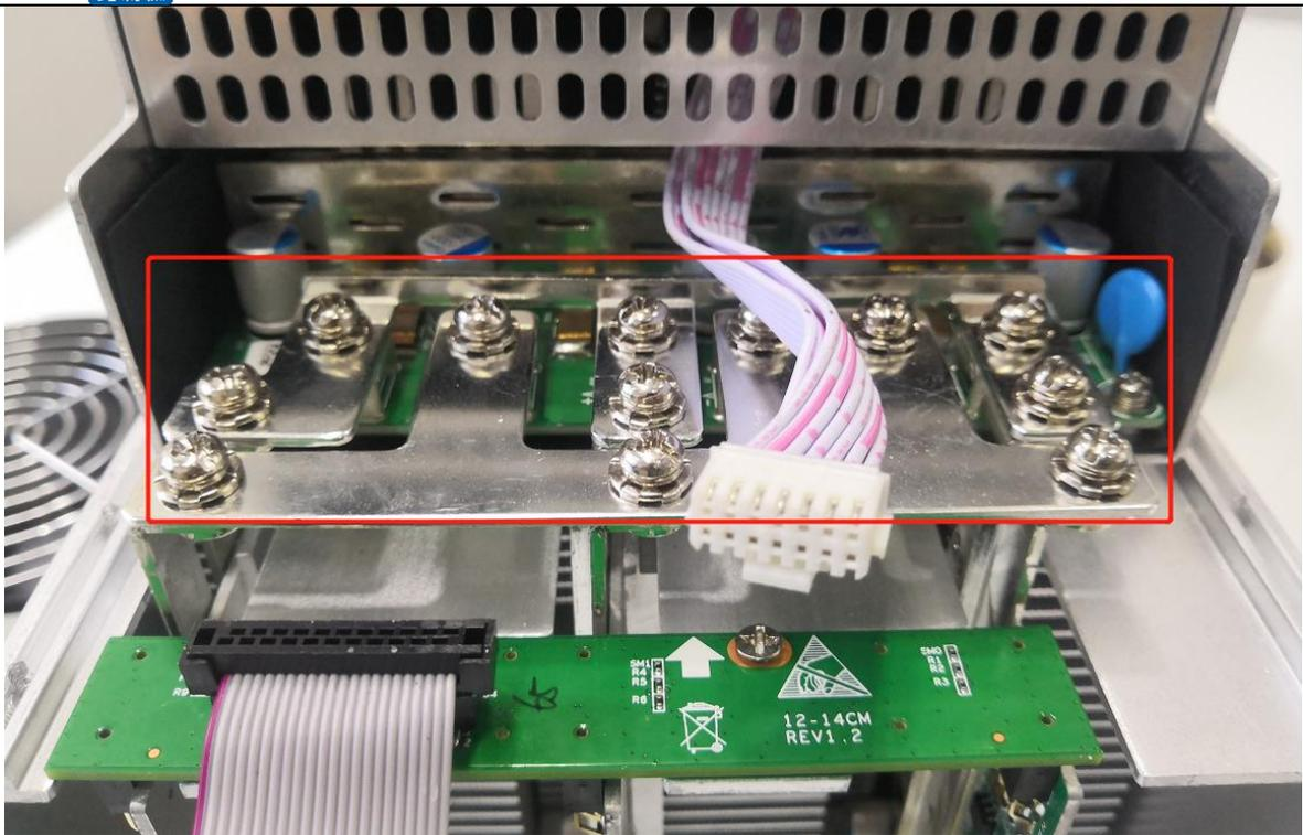
4) After the copper row is installed, the control board and the fan are installed, and the hash board is installed.
