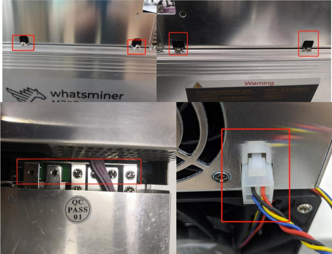
2) After the above operation is completed, gently pull out the power supply (do not pull out too long, the power control cable is still connected to the control panel), as shown in the figure:
