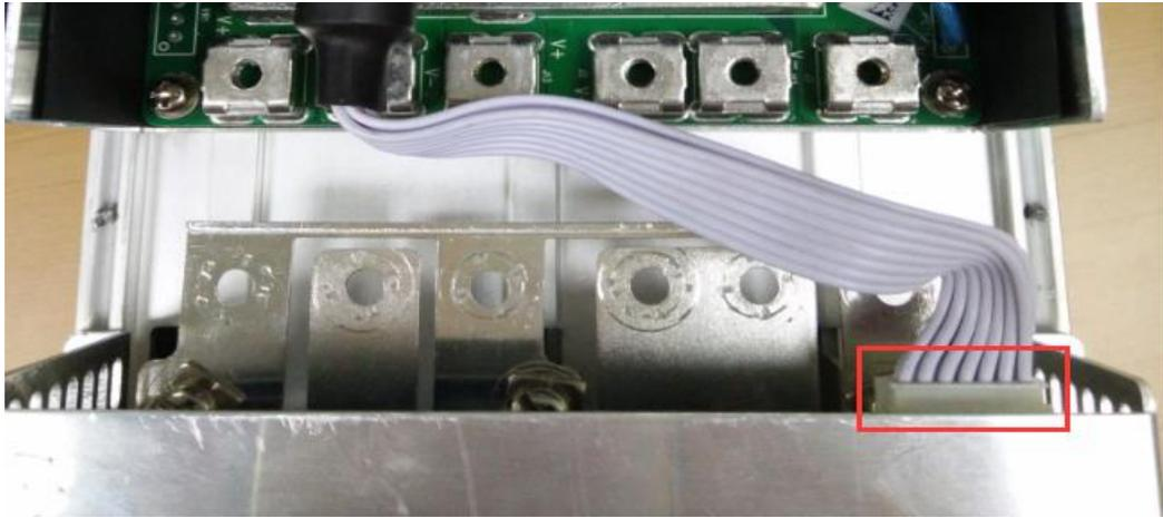
2) Then connect the 6 positive and negative terminals on the power supply to the copper row one by one, and then install 6 screws in turn. The screws should be tightened and the washers should be aligned parallel to the edge of the copper bar to avoid short circuiting the power supply or the power board, as shown below:
